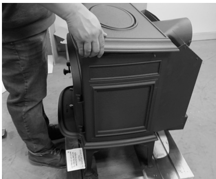
Fig.6.5. Remove the top plate from stove.
