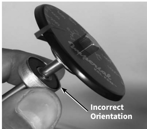
Fig. 5.6. Remove magnet from current orientation
