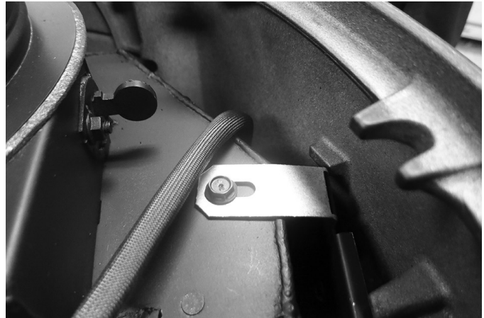
Figure 16.2. Remove the firebox-to-side plate bolt.
